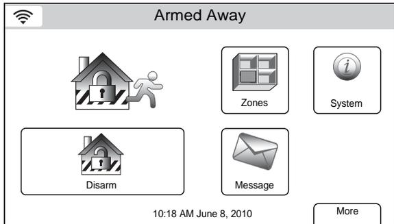
4. At the end of the exit delay the system will announce "Armed Away" and displays the "Armed Away" screen.
