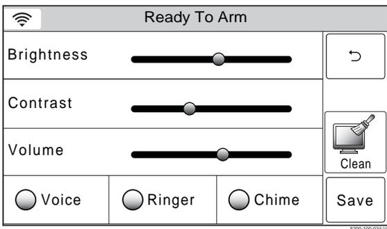
2. Increase or decrease the Display Brightness or Contrast or the System Volume by using the sliding adjustment from left (decrease) to right (increase).
