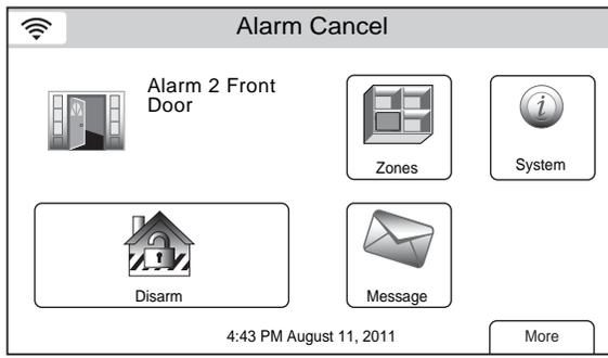
2. “Alarm Cancel” is displayed in a red band along with the zone that caused the alarm. Select the “Disarm” icon and enter an second Off sequence to clear the alarm. The system beeps once, returns to the Security Screen and announces “Disarmed Ready to Arm”.
