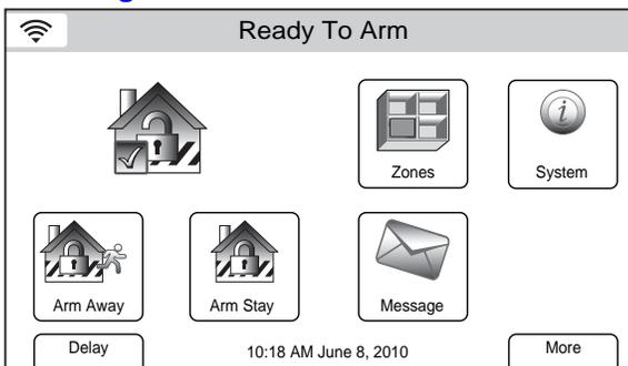
1. With the system in the disarmed state, select the “Zones” icon from Security Screen. The system displays the Zones screen.
