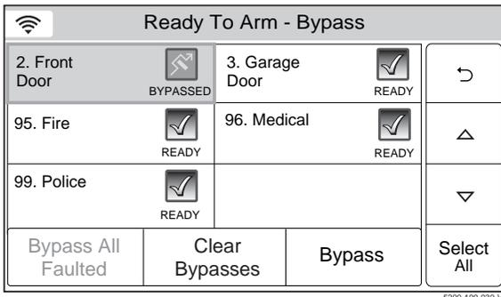
4. To clear the bypass, select the **bypassed zone(s)**, then select the “Clear Bypasses” button.
