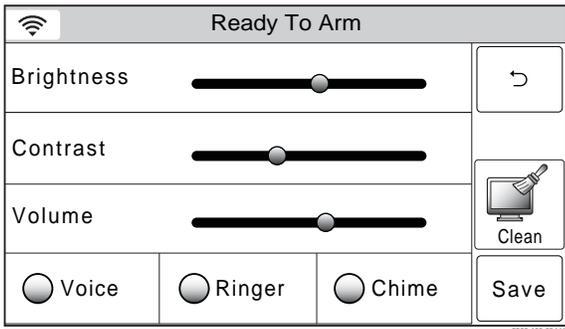
2. Select the “Chime” icon. The system toggles between “Off” and “On” and when selected the button turns green. When “On” is selected, the Chime mode will be active.
