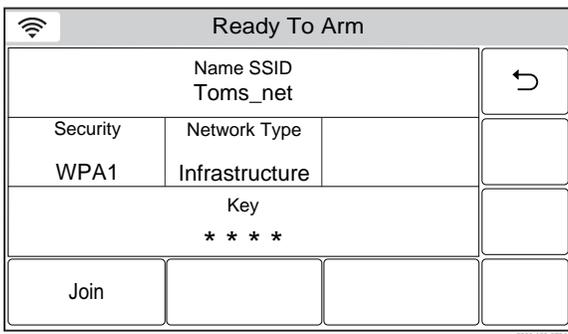
3. Select the “SSID Name” button and enter Network name on the displayed keypad.
