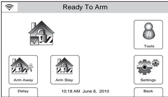
1. With the system in the disarmed or armed state, select the "Settings" icon from the second page of the Security Screen. The system displays the Settings screen.
