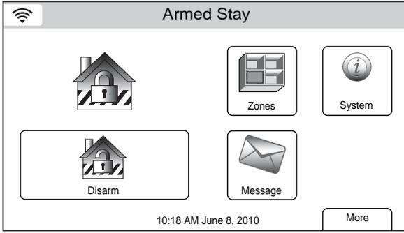
4. At the end of the exit delay the system announces "Armed Stay" and displays the "Armed Stay" screen.
