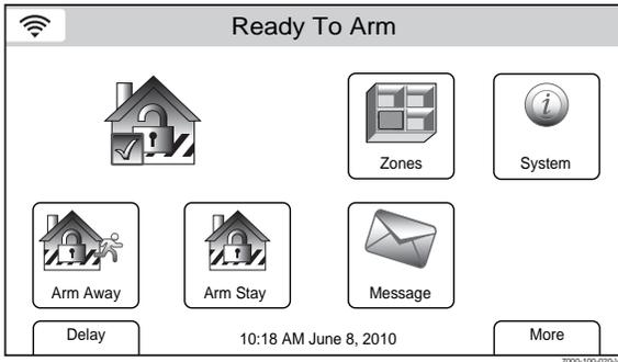
1. With the system in the disarmed state, select the “Zones” icon. The system displays the Zone screen and the status for each zone will be indicated.
