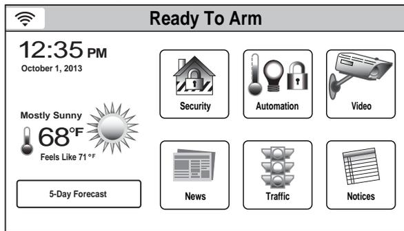
1. With the system in the disarmed state, select the "Automation" icon from the Home Screen. The system displays the first page of the Automation screen. Select the select the "▼" icon to advance to the second page of the Automation screen.
