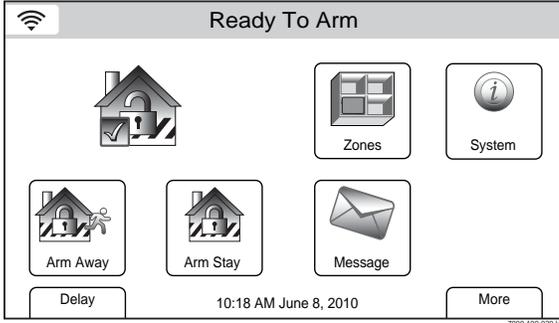
1. With the system in the disarmed state, select the “Message” icon from the Security Screen. The system displays the Message screen.
