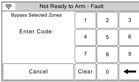
3. Enter a valid Code. The system returns to the Bypass screen and the zone(s) that are bypassed will be displayed.
