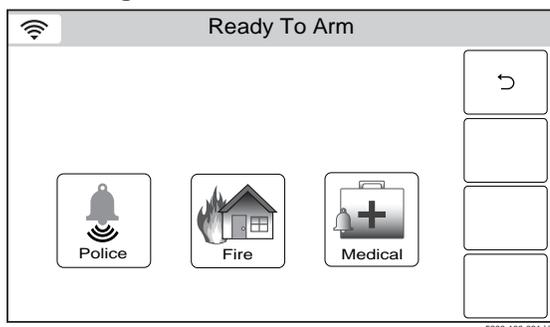
1. With the system in the disarmed or armed state, depress and hold the “Panic” key until the system displays the Panic screen (approximately 3-4 seconds).
