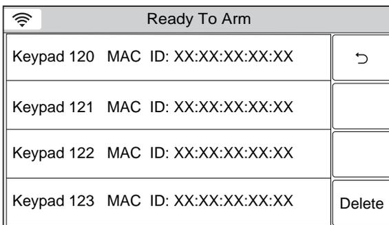
2. To delete a **mobile device** (auxiliary keypad) select the keypad to be deleted.
