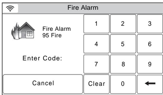
**Note:** Dependent upon how your system has been programmed a keypad may be displayed. This will allow you to cancel the alarm by entering valid User Code on the keypad.
