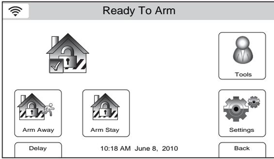
1. With the system in the disarmed state, select the “Settings” icon from the second page of the Security Screen. The system displays the Settings screen.
