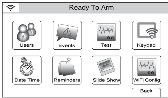
3. Select the “Test” icon. The system displays the Test screen.
