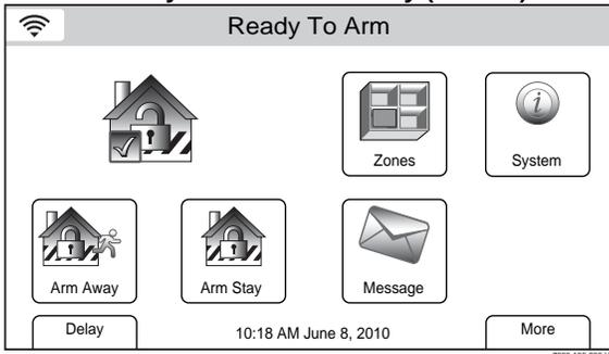
1. Select the “Delay” tab on the Security Screen. The icon “toggles” and “Instant” is displayed.
