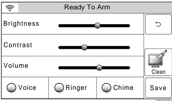
2. Select the "Voice" icon. The system will toggle between "Off" and "On" and when selected the button turns green. When "On" is selected, the Voice mode will be active.
